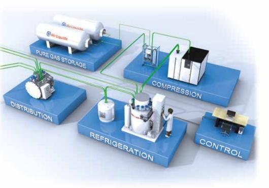
ir Liquide designs and manufactures the closeloop refrigeration system necessary to cool down the moderator fluid.
